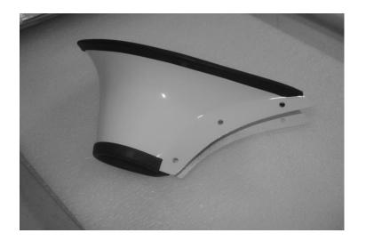
Once the fiberglass is trimmed to fit the body, the 1/4" channel can be cut and fit to shorts.
